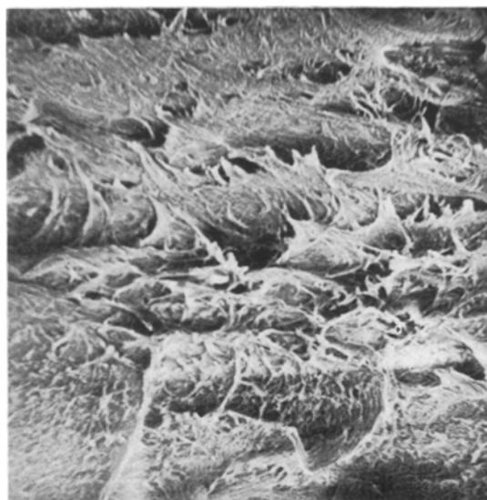
Figure 13 Micrograph of the fracture surface of a polypropylene specimen of birefringence 0.015, \times 830 .
