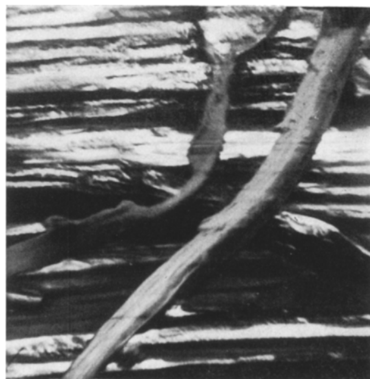
Figure 14 Fracture surface of a polypropylene specimen taken from the neck region, \times 1620 .
